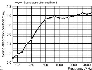
$<sup>^{\</sup>rm o}$  Equivalent sound absorption area less than 1.0 m²  $\alpha_{\rm S}$  Sound absorption coefficient according to ISO 354
