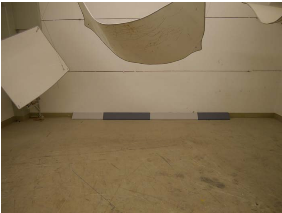
Figure B.2. Set-up of the edge elements in room edge 2 in the reverberation room (overall length 4000 mm).
