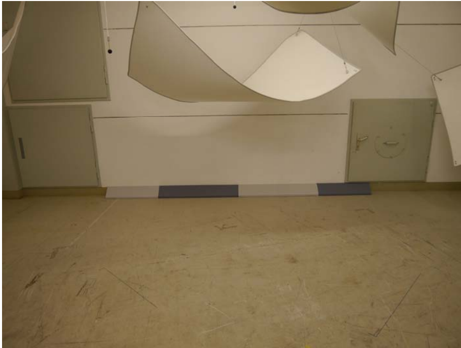
Figure B.1. Set-up of the edge elements in room edge 1 in the reverberation room (overall length 4000 mm).
