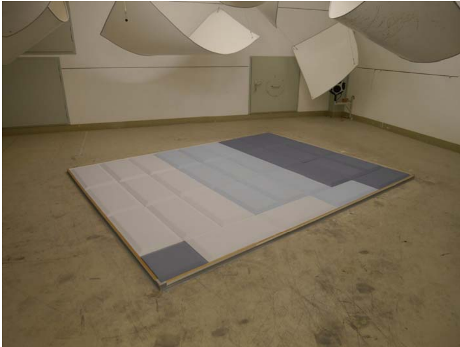
Figure B.1. Set-up of the wall panels in the reverberation room.
