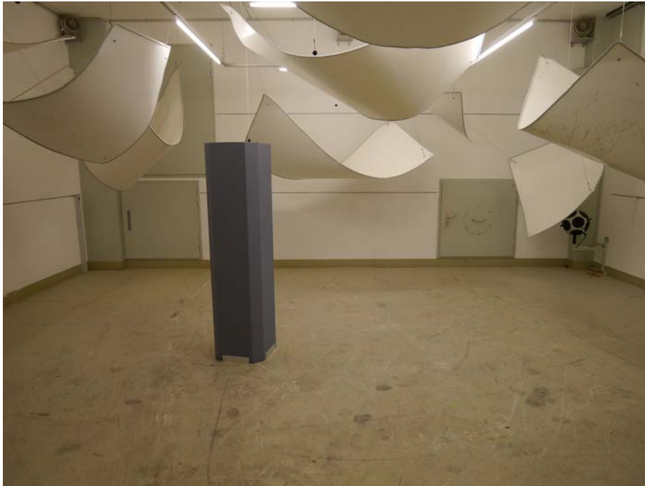
Figure B.1. Set-up of the column in the reverberation room (one out of five positions in total).
