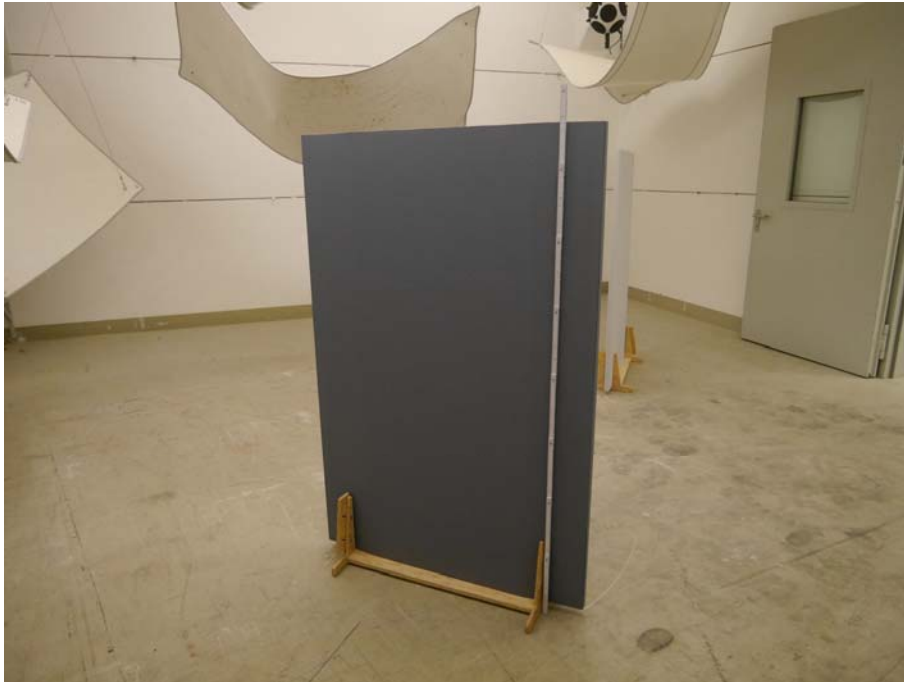
Figure C.3. Set-up on the floor of the reverberation room.
