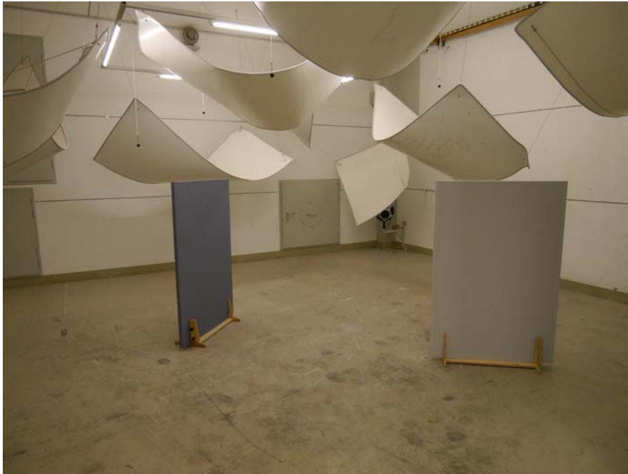
Figure C.1. Set-up of the room dividing partitions in the reverberation room.
